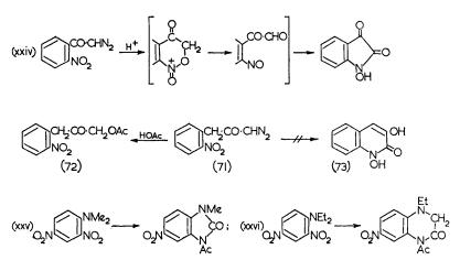
Among derivatives of *o*-nitroaniline a remarkable type of interaction<sup>90</sup> is represented by the reactions (xxv) and (xxvi) which are effected by zinc chloride in hot acetic anhydride. Acid-catalysed cyclisation of 2-nitro-hydrazobenzenes has already been mentioned (p. 399; ref. 42) and operates in the formation<sup>91</sup> of benzotriazole derivatives from 4-alkyloxybutan-2-ones and 2,4-dinitrophenylhydrazine in presence of hydrochloric acid.
