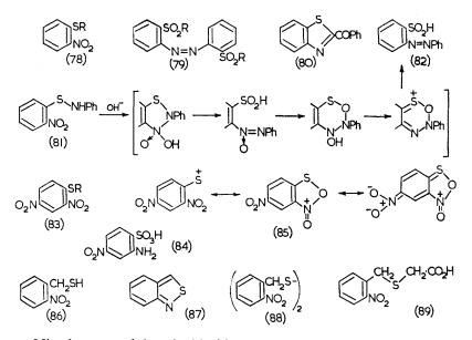
o-Nitrobenzenesulphenyl chloride (78; R = Cl) also reacts in hot aqueous methanol to form orthanilic acid (84; H for NO<sub>2</sub>),<sup>120</sup> and in a vigorous reaction with hydrogen fluoride yields the azobenzenesulphonyl fluoride (79; R = R = F) among other products.<sup>121</sup> According to Kaluza and Perold<sup>122</sup> the reaction (83;  $R = Cl) \rightarrow (84)$  in boiling acetic acid requires activation by light and proceeds through the hydroxylamine (84:
